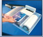
Place the corner of the product on the combination film separator/loading table. Slide the product into the open end of the center-fold film, and into the sealing position. The leading edge of the film was left sealed when the previous package was made.
