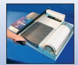
With the film covered product now resting on the work table, close the sealing jaw to form a bag around the product. Product is now in a bag with one open end, and the edge of the film is sealed for the next package.
